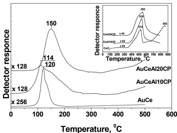
Fig. 1. TPR spectra of the gold-based catalysts; inset: initial supports.
