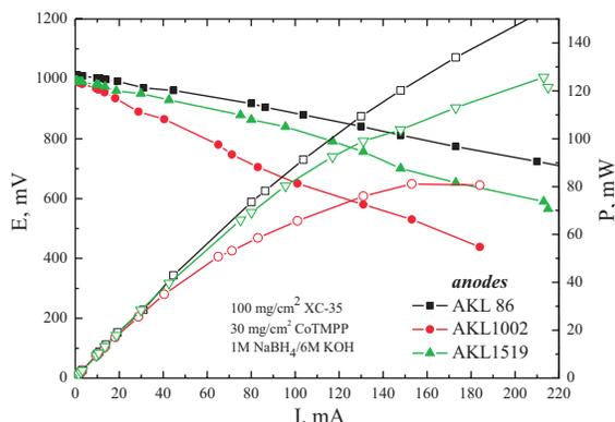
**Fig. 4.** Polarization and power characteristics of a borohydride fuel cell
