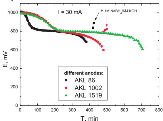
**Fig. 5.** Discharge curves of the experimental fuel cell.
