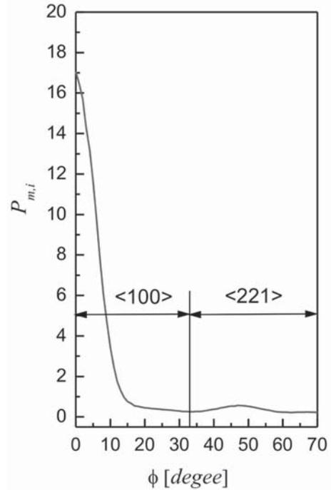
**Fig. 2.**  $\{200\}$  pole figure of an electrodeposited nickel (Ni1) measured at generator current  $i$ . It represents the distribution of strongly extinction-affected pole densities:  $P_{m,i}(\phi) = I_{m,i}(\phi) / I_{m,i}^r$ ,  $\phi$  is the angle to the sample normal direction.
