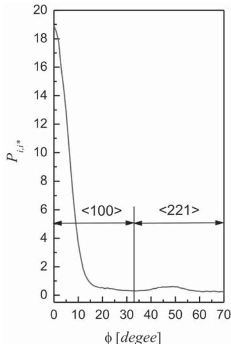
**Fig. 4.** {200} pole figure of an electrodeposited nickel coating (Ni1) representing extinction-free data calculated by (16).
