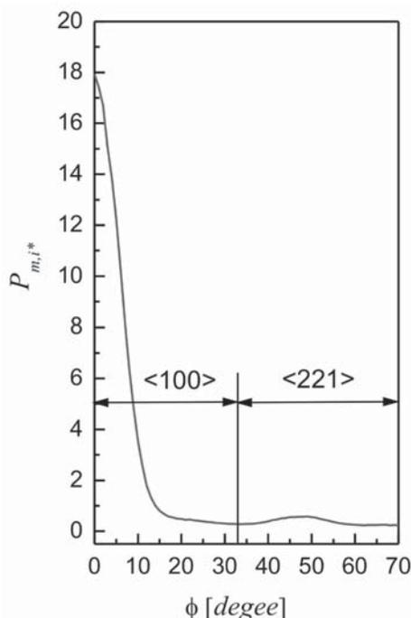
**Fig. 3.** {200} pole figure of an electrodeposited nickel coating (Ni1) measured at generator current  $i^*$ . It represents the distribution of less extinction-affected pole densities:  $P_{m,i^*}(\phi) = I_{m,i^*}(\phi)/I_m^r$
