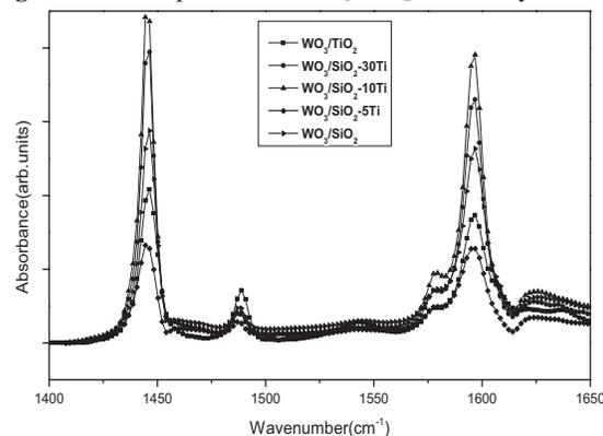
Fig3. The FT-IR spectra of pyridine adsorbed on various samples at 50°C.
