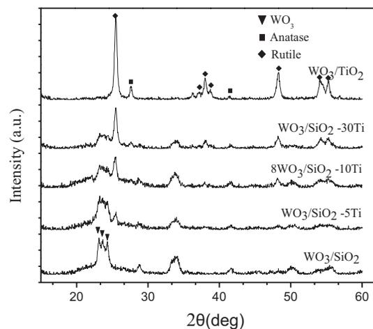
Fig.2. The XRD patterns of WO<sub>3</sub>/SiO<sub>2</sub>-xTi catalysts.
