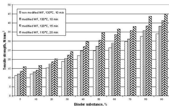
**Fig. 4.** Tensile strength as a function of BS%
