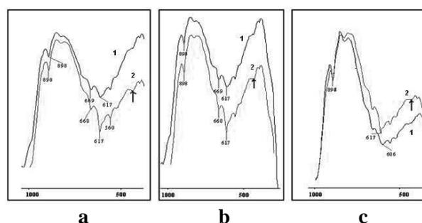
**Fig. 1.** IR spectrum of: a) non-modified (1) and modified (2) wood flour with system of three components (40% addition based on wood flour); b) non-modified (1) and modified (2) wood fibers with system of two components (30% added based on wood fibers); and c) non-modified (1) and modified (2) wood fibers with system of two components (40% added based on wood fibers).
