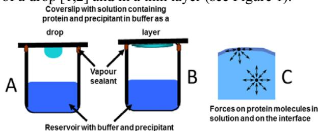
**Fig. 1.** Hanging drop crystallization set-up: **A.** in the classical (drop), and **B.** new modified variant (layer). **C.** Protein molecules in the bulk and on the interface. Intermolecular forces that arise between two equal molecules are demonstrated by arrows.
