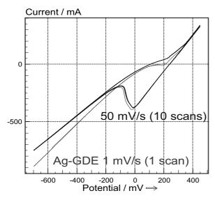
**Fig. 8.** CV measured during oxygen reduction on Ag-GDE in 10 N NaOH at 80°C with scan rates of 50 mV/s and 1 mV/s.
