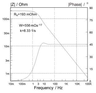
Fig. 19. Bode diagram of simulated impedance spectra of the Nernst impedance  $Z_N$  with  $\,W\!\!=\!\!556~m\Omega s^{\text{-}1/2}$  and  $k_N\!\!=\!8.33~s^{\text{-}1}.$
