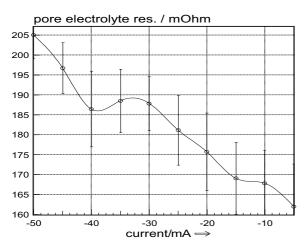
**Fig. 16.** Current density dependence of the pore electrolyte resistance during oxygen reduction reaction on Ag-GDE in 10 N NaOH, 80°C.
