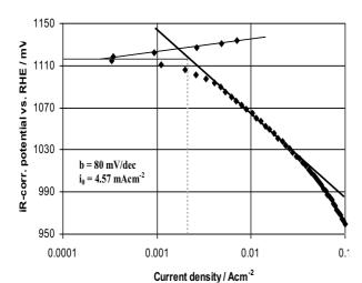
**Fig. 10.** Tafel-plot of data measured during ORR on Ag-GDE in 10 N NaOH at 80°C.
