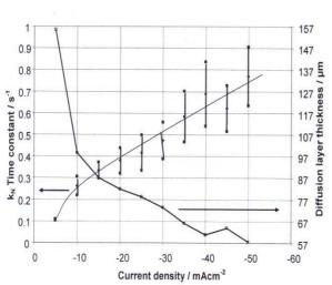
**Fig. 18.** Current density dependence of the diffusion time constant ( $2^{nd}$  parameter of  $Z_N$ ) and calculated diffusion layer thickness during oxygen reduction reaction on Ag-GDE in 10 N NaOH, 80°C.
