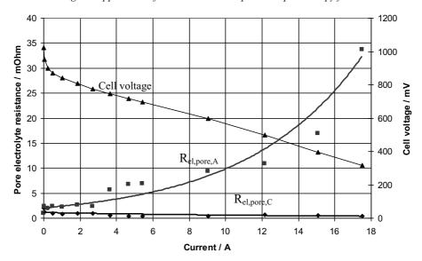
Fig. 6. Current dependence of cell voltage ( $\triangle$ ), pore electrolyte resistance of the anode ( $R_{el,pore,A}$ ) ( $\blacksquare$ ) and cathode ( $R_{el,pore,C}$ ) ( $\spadesuit$ ).
