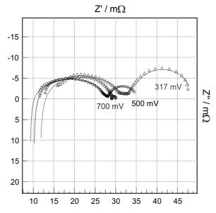
**Fig. 3.** Nyquist diagram of selected EIS measured on PEFC at low cell voltages, 80°C, at 2 bar absolute, at different cell voltages (currents): (o) 700 mV (5.4 A), ( $\square$ ) 500 mV (12.1 A) and ( $\Delta$ ) 317 mV (17.5 A).
