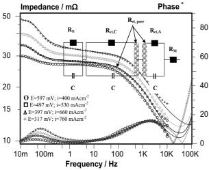
**Fig. 4.** Bode diagram of EIS measured in the low cell voltage range, at 80°C, at 2 bar absolute, at different cell voltages (currents): (o) 597 V, ( $\square$ ) 497 mV, ( $\Delta$ ) 397 mV and (+) 317 mV with the schematic representation of the used EC for fitting as insert.
