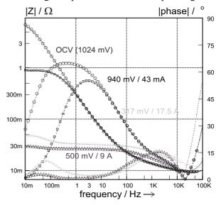
**Fig. 2.** Bode diagram of selected EIS measured on PEFC,  $80^{\circ}$ C, at 2 bar absolute, at different cell voltages (currents): (o) 1024 V, ( $\square$ ) 940 mV, ( $\Delta$ ) 500 mV and (+) 317 mV.
