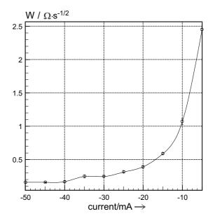
**Fig. 17.** Current density dependency of the Warburg parameter (W) during oxygen reduction reaction on Ag-GDE in 10 N NaOH, 80°C
