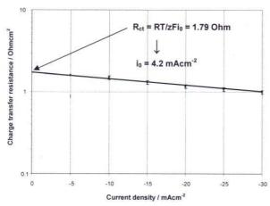
**Fig. 14.** Low current density dependence of the charge transfer resistance (logarithmical representation) during oxygen reduction reaction on Ag-GDE in 10 N NaOH, 80°C.
