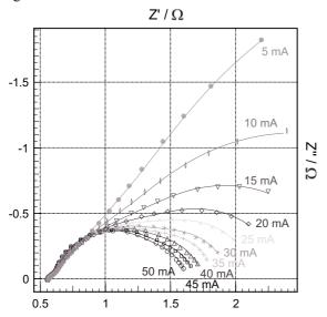
**Fig. 12.** Nyquist representation of impedance spectra measured in the frequency range from 50 mHz to 10 kHz at different current densities during oxygen reduction reaction on Ag-GDE in 10 N NaOH
