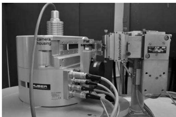
Fig. 1. Swinging flat sample setup
