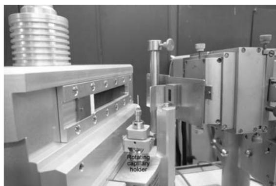
Fig. 2. Rotating capillary setup
