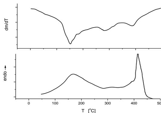
**Fig. 1.** Results of TG and DSC studies of the samples with 10 % Ni content at heating rates of 20 [K/min]. The top of the figure is the mass derivative as a function of temperature. The bottom presents the DSC scan.
