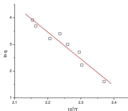
**Fig.2.** Arrhenius plot of the dependence of temperature of the reciprocal of the maximum of the first endothermic peak,  $T_{\text{max}}$  [K], on the heating rate,  $q$ .
