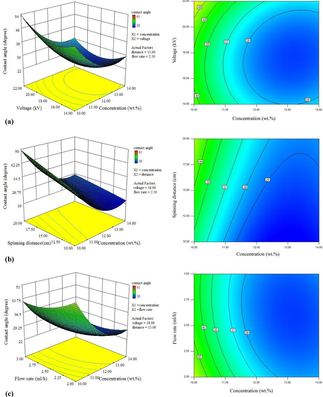
**Fig. 10.** Response surface and contour plots of CA showing the effect of: (a) solution concentration and applied voltage, (b) solution concentration and spinning distance, (c) solution concentration and volume flow rate.
