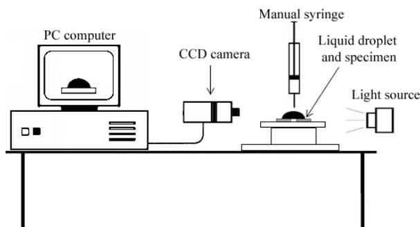
Fig. 2. Schematic of contact angle measurement set up.
