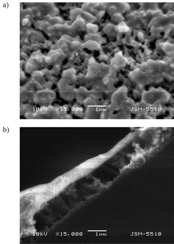
**Fig. 2.** SEM images of 20SiO<sub>2</sub>-80ZnO films: (a) top view of the coatings surface morphology; (b) cross section of the nanocomposite film
