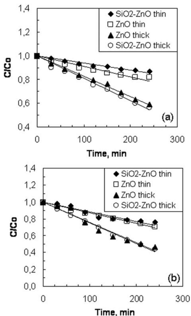
**Fig. 5.** Comparison of the photodegradation kinetics of malachite green with the photocatalytic films under catalytic action under: (a) UV irradiation and (b) visible light. The initial MG concentration is 5 ppm
