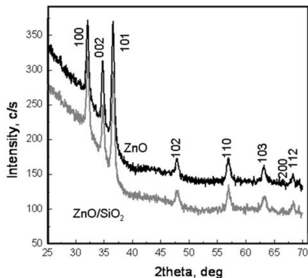
**Fig. 3.** Comparative XRD of ZnO and ZnO-SiO<sub>2</sub> composite films
