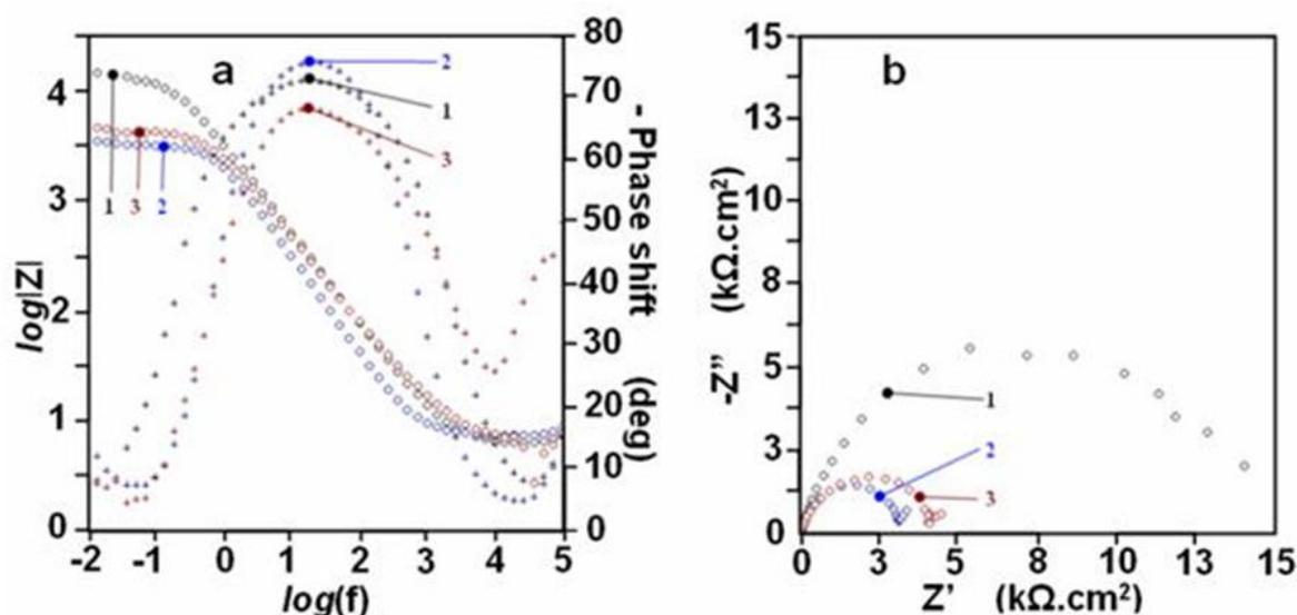
**Fig. 1.** Bode (a) and Nyquist (b) plots of the EI-spectra of three samples of Group 6. 1 – sample P1; 2 – sample P2; 3 – sample P3
