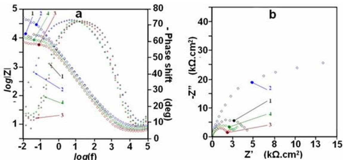
**Fig. 2.** Bode (a) and Nyquist (b) plots of the EI-spectra of CeCC coatings deposited after mechanical pretreatment and different  $H_2O_2$  additions: 1 – sample P1, after 48 hours of exposition; 2 – sample P5 after 48 hours of exposition; 3 – sample P1 after 168 hours of exposition; 4 - sample P5 after 168 hours of exposition
