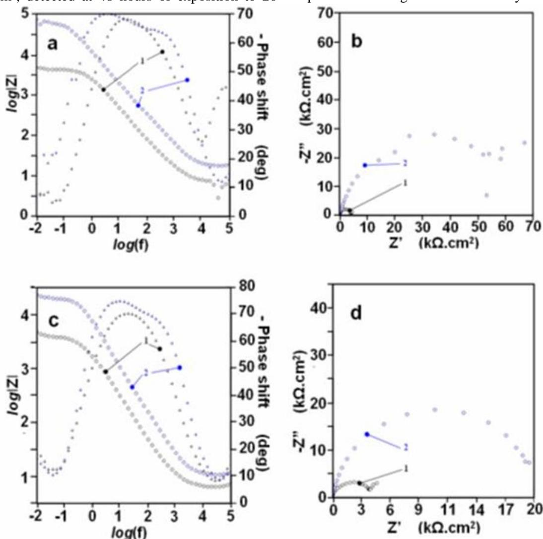
**Fig. 3.** Electrochemical Impedance Spectra recorded after 48 (a) and 168 (b) hours of exposure of two samples with different pH of the coating solutions. 1 – specimen P3; 2 – specimen P4.
