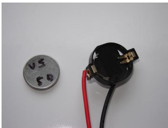
**Fig. 5.** Li-Air button cell 2032 and holder
