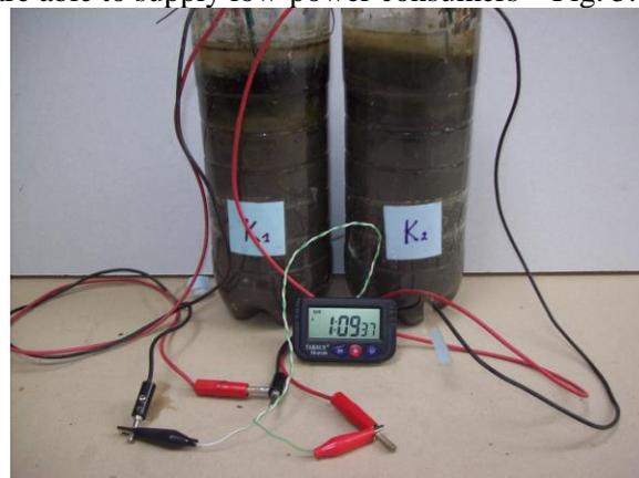
**Fig. 5.** Connected in series SMFCs supplying digital watch
