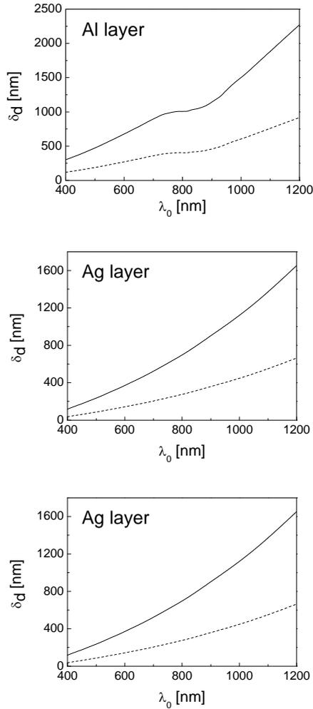
**Fig. 3.** Dependence of the SPP penetration depth in the dielectric on the wavelength for Al, Au and Ag layer. The dielectric is air (solid line) or polycarbonate (dashed line).
