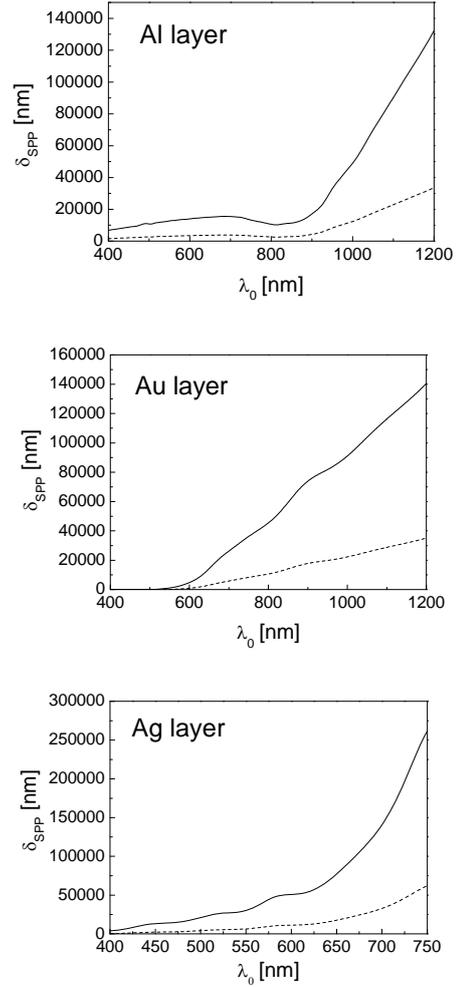
**Fig. 2.** Dependence of the SPP propagation length on the wavelength for Al, Au and Ag. The dielectric is air (solid line) or polycarbonate (dashed line).
