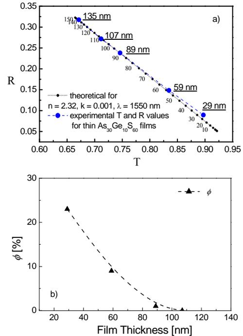
**Fig. 4.** Theoretical R-T dependence for thin  $\text{As}_{30}\text{Ge}_{10}\text{S}_{60}$  films and experimental data for thin  $\text{As}_{30}\text{Ge}_{10}\text{S}_{60}$  films (a). The parameters of the theoretical line are given in the graphs. Porosity  $\phi$  vs. film thickness (b).
