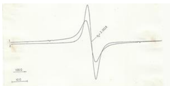
Fig. 1. ESR signal of standard activated carbon and of coke on the catalyst
