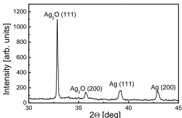
Fig. 2. X-ray diffraction pattern of thin Ag-PMMA film.
