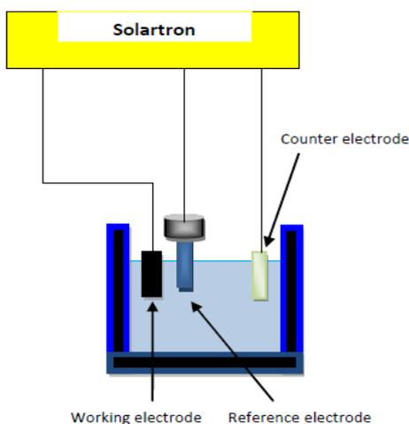
Fig.1. Three-electrode cell
