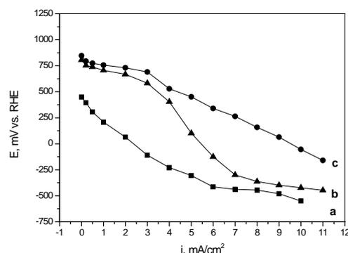
**Fig. 4.** Polarization curves for electrodes from teflonized Vulcan XC-72 and DG + 20 % CoPc, in different electrolytes: a – electrolyte 1 %  $\text{SO}_2$  + 18 g/l NaCl; b - electrolyte 1 %  $\text{SO}_2$  + 1 M NaOH; c - electrolyte 1 %  $\text{SO}_2$  + 18 g/l NaCl + 1 M NaOH.
