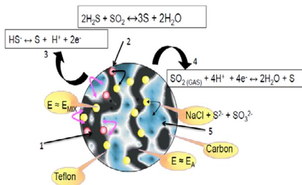
**Fig. 6.** Physical model of the pore of a micro galvanic element with teflonized charcoal /carbon black and catalytic mass for reduction reaction of  $\text{SO}_2$  with the oxidation of  $\text{H}_2\text{S}$  in the electrolyte (1%  $\text{SO}_2$  + 18 g/l  $\text{NaCl}$  + 1 M  $\text{NaOH}$  +  $\text{Na}_2\text{S} \cdot 9 \text{H}_2\text{O}$ ).
