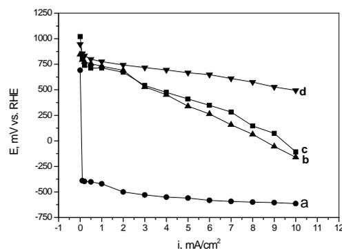
**Fig.3.** Polarization curves of sulfur dioxide reduction in aqueous electrolyte:  $\text{SO}_2$  1% vol. +1 M NaOH + 18  $\text{g.l}^{-1}$  NaCl. Tested electrodes are: a - type network (stainless steel); b - 35% teflonized Vulcan XC-72 and DG +20% CoPc; - perovskite; d - 35% teflonized Vulcan XC-72 and DG +20% CoPc + 6% Pt.
