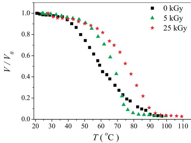
Fig. 7. Temperature surface potential decay curves for negatively charged non-irradiated and gamma irradiated PP films.
