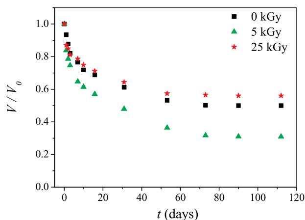
Fig. 2. Time dependences of the normalized surface potential for positively charged non-irradiated and gamma irradiated PP films.
