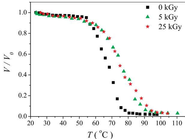
Fig. 9. Temperature surface potential decay curves for negatively charged non-irradiated and gamma irradiated PET films.
