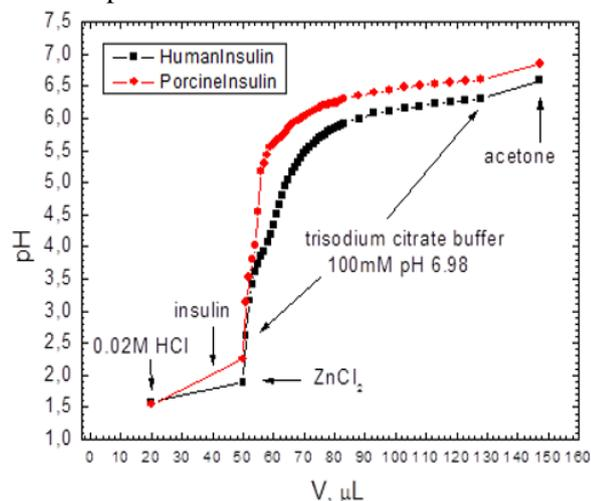
**Fig. 3.** Titration curves of insulin (porcine and human) dissolved in HCl solution with citric buffer.
