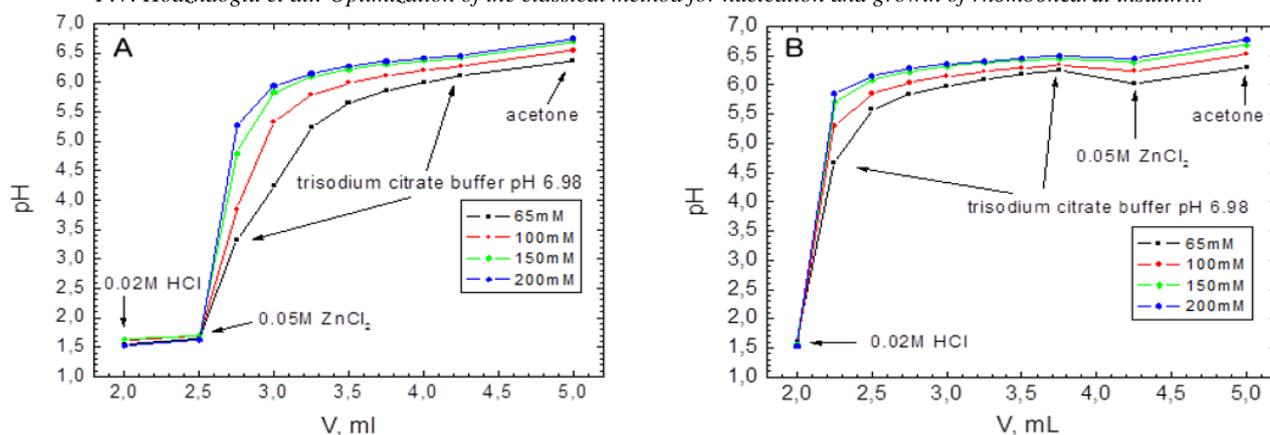
**Fig. 2.** Titration curves of hydrochloric acid solution with citrate buffer in presence of zinc chloride (A) or adding the zinc chloride before the acetone (B). The incorporation points of zinc chloride and acetone are indicated with arrows. The titration interval with citrate buffer is flanked with two arrows.
