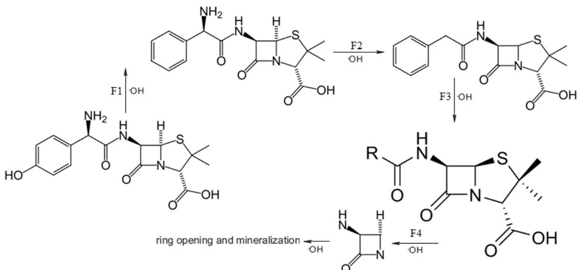
**Fig. 2.** Possible pathways for the photocatalytic degradation of amoxicillin.
