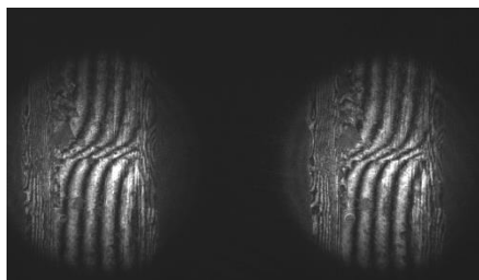
Fig. 2. Spatially shifted patterns, imaged on the CCD camera plane.
