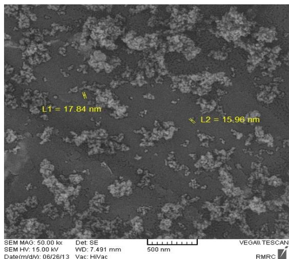
**Scheme 1.** SEM image of HBF<sub>4</sub>-SiO<sub>2</sub> NPs
