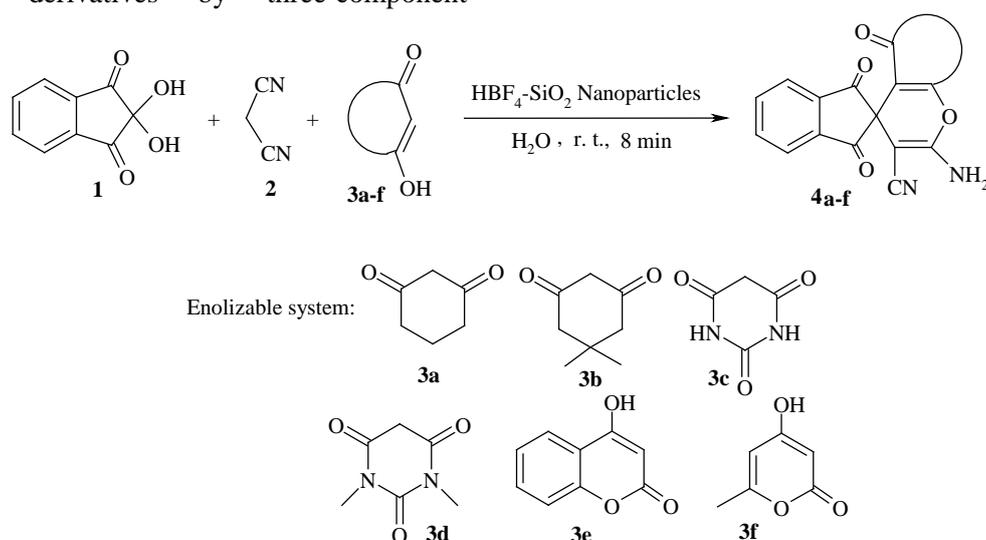
**Scheme 2.** Synthesis of spiro-2-amino-4H-pyran-3-carbonitrile derivatives catalyzed by HBF<sub>4</sub>-SiO<sub>2</sub> NPs.
