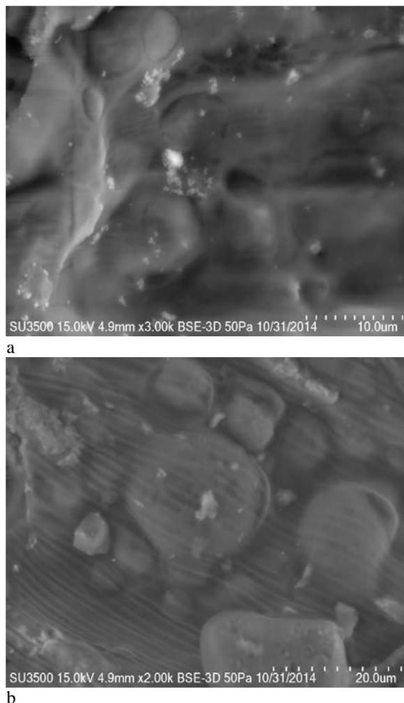
**Fig. 4.** SEM of TiO<sub>2</sub> nanoparticles from water extract of *A. anthodium* a) the scale bar is 10 μm, b) the scale bar is 20 μm
