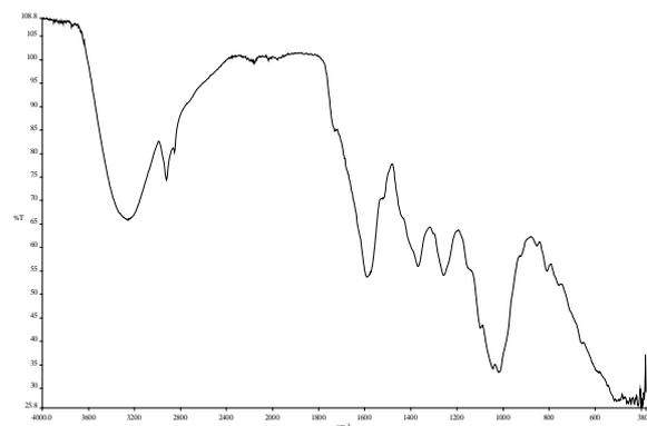
**Fig. 2.** FTIR spectrum of TiO<sub>2</sub> nanoparticles from water extract of *A. anthodium*
