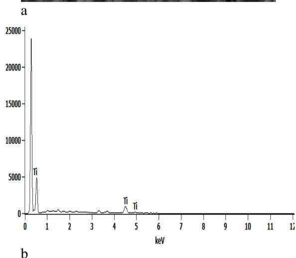
**Fig. 5.** a) SEM and b) EDS profile of TiO<sub>2</sub> nanoparticles from water extract of *A. anthodium*
