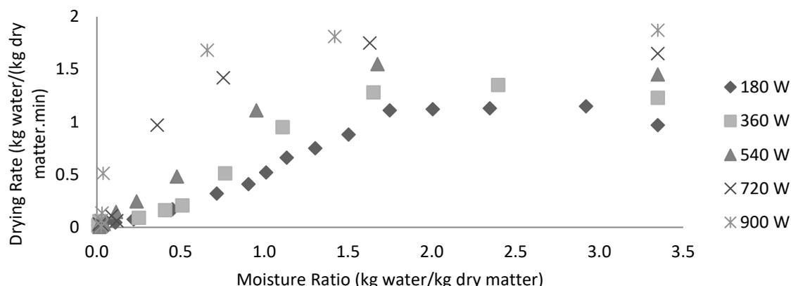
**Fig. 1.** Variation of the drying rate (kg water / (kg dry matter min<sup>-1</sup>) as a function of the moisture ratio (kg water/kg dry matter) for different microwave powers.
