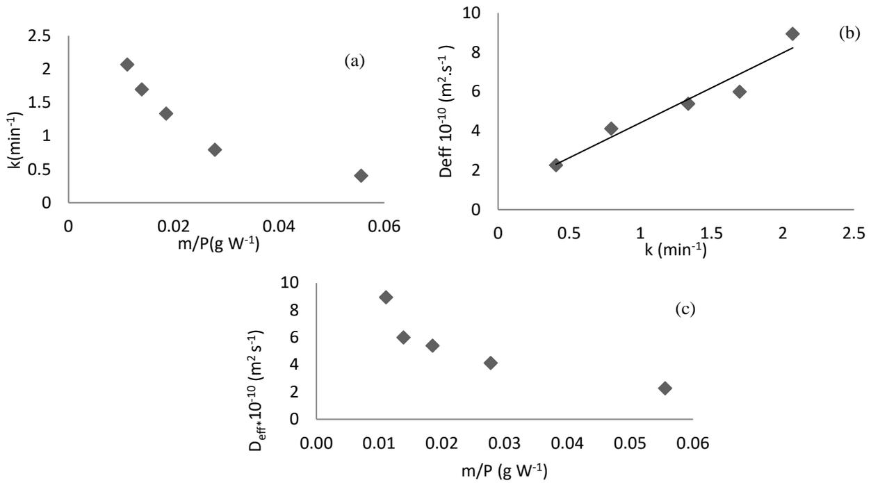
**Fig. 3.** (a) Relationship between the drying rate constant ( $k$ ) of Page model and the sample mass /power ratio, (b) Relationship between the drying rate constant ( $k$ ) and the effective moisture diffusivity ( $D_{\text{eff}}$ ) for microwave drying of corn husks (■ calculated data; - model), (c) Relationship between the effective moisture constant and the sample mass.
