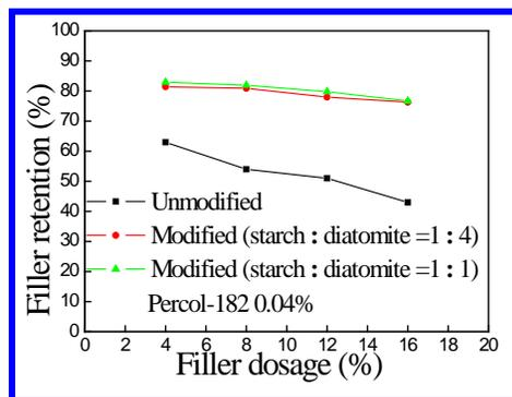
Fig. 7. Effect of filler dosage on filler retention.
