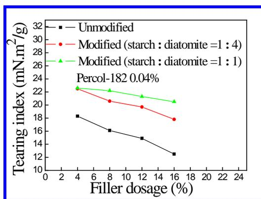
Fig. 5. Effect of filler dosage on the tearing index of filled handsheets.
