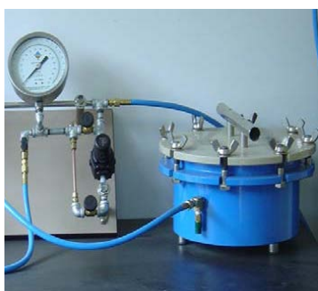
Fig. 1. Pressure plate test device
