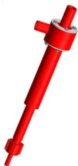
Fig. 5. The general cyclone
