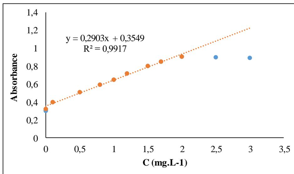
**Fig. 8.** The calibration curve for 10 ml CPZ aqueous solution with concentration of the 0.005 to 2  $\mu\text{g}.\text{ml}^{-1}$  range pH=10, organic solvent: methanol, extraction time: 16 minutes, the Nanoparticle amount: 40mgr , desorption time:5 minutes and salt: 5% W/V .
