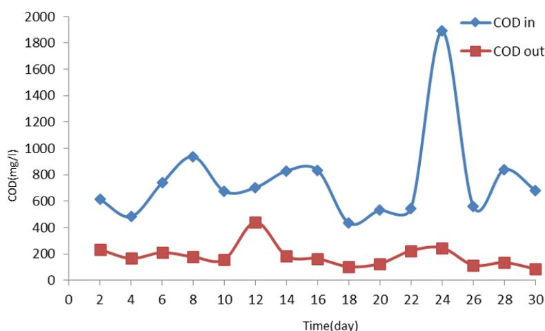
**Fig. 2.** Variation of influent and effluent COD versus different days.
