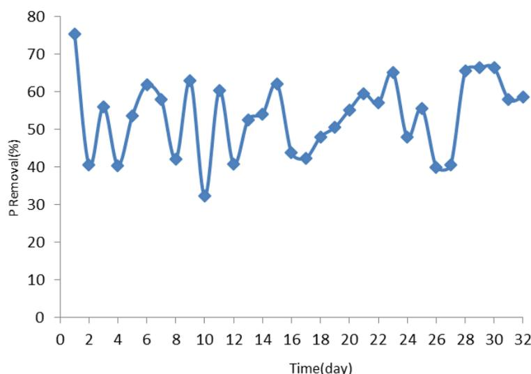
Fig. 5. TP removal efficiency in different operational days.
