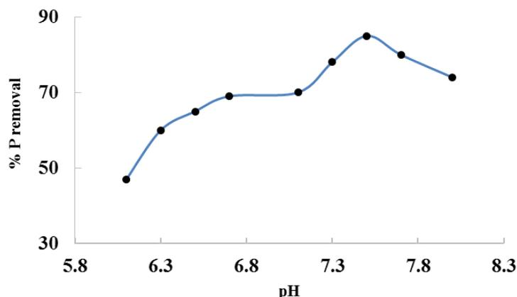
**Fig. 7.** Effect of pH on removal efficiency of TP.
