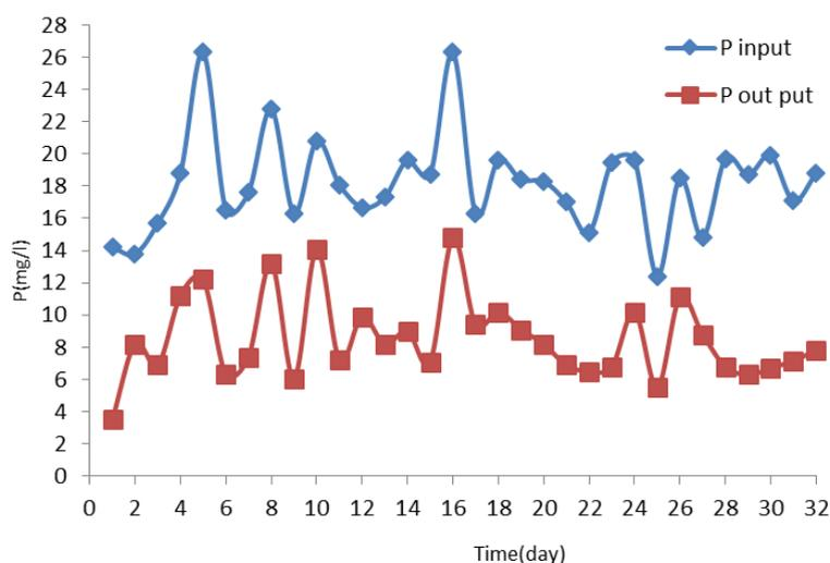
Fig4. Variation of influent and effluent TP versus different days.
