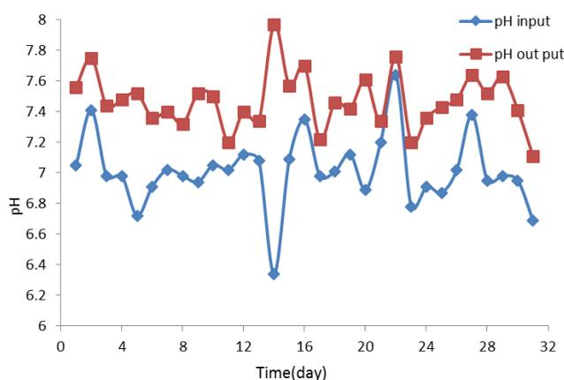
**Fig. 6.** Influent and effluent wastewater pH in different operational days.
