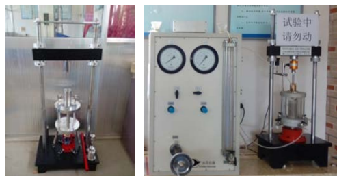
Fig. 1. Triaxial test apparatus for unsaturated soils and sampling devices
