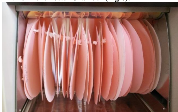
Fig. 6 Paper samples in the Suntest apparatus
