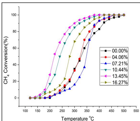
**Figure 1.** Temperature dependence of methane conversion over different amounts of gold loaded on 18wt.% Co/ $\gamma$ -Al<sub>2</sub>O<sub>3</sub>.
