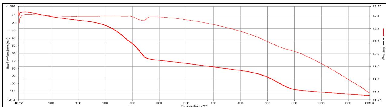
Figure 5. Graphical representation of TGA/DSC thermograms of the precursors of 10.44wt.% Au supported on 18wt.%Co/ $\gamma\text{-Al}_2\text{O}_3$
