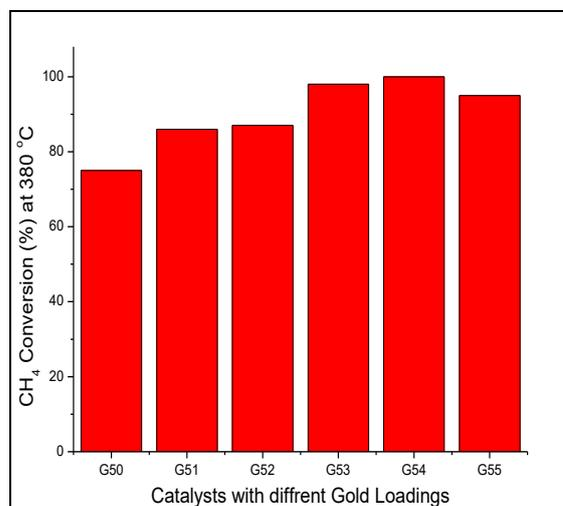
**Figure 2.** Methane conversion at 380°C for all catalysts.
