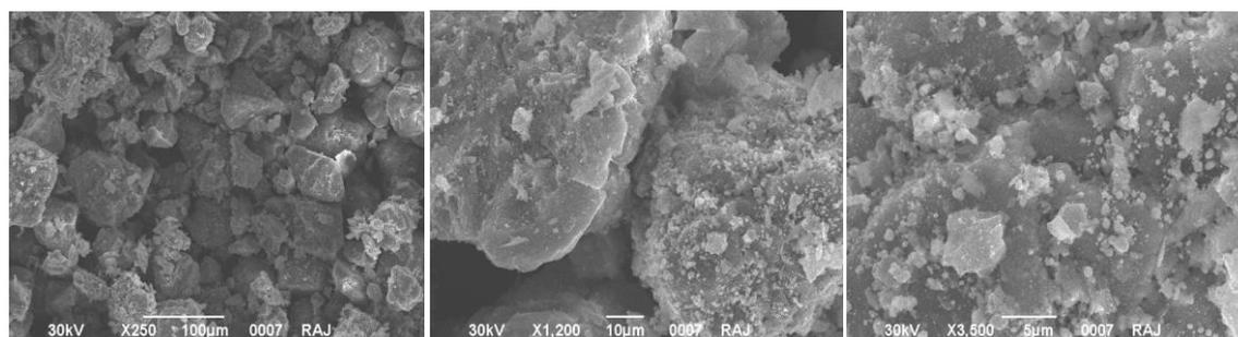
**Figure 8.** SEM micrographs of G52 catalyst.
