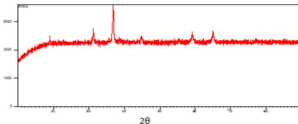
Figure 4. XRD pattern of 18wt.% Co/ $\gamma\text{-Al}_2\text{O}_3$
