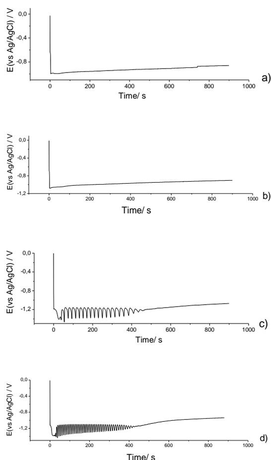
**Fig. 6.** Chronopotentiometric curves obtained at different current densities at  $\text{pH}=3.5$ .  $C_{Sn} = 5 \text{ g dm}^{-3}$ ;  $C_{Co} = 5 \text{ g dm}^{-3}$ . a)  $0.8 \text{ A dm}^{-2}$ , (b)  $1.0 \text{ A dm}^{-2}$ , (c)  $1.6 \text{ A dm}^{-2}$ , (d)  $2.0 \text{ A dm}^{-2}$
