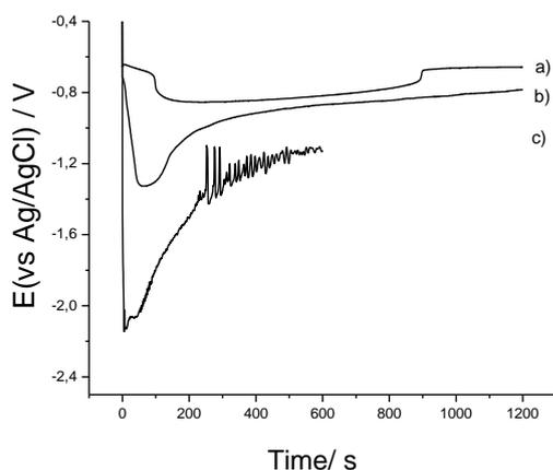
**Fig. 3.** Chronopotentiometric curves obtained at different current densities at  $\text{pH}=3.5$ .  $C_{Sn} = 10 \text{ g dm}^{-3}$ ;  $C_{Co} = 0 \text{ g dm}^{-3}$ . (a)  $0.4 \text{ A dm}^{-2}$  (b)  $0.6 \text{ A dm}^{-2}$  (c)  $1.6 \text{ A dm}^{-2}$
