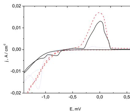
**Fig. 1.** CVA curves of tin, cobalt and SnCo alloy deposition from sulphate/gluconate electrolytes at pH=5. C<sub>Na<sub>2</sub>SO<sub>4</sub></sub> = 40 g dm<sup>-3</sup>; C<sub>C<sub>6</sub>H<sub>11</sub>NaO<sub>7</sub></sub> = 50 g dm<sup>-3</sup>; v = 20 mV s<sup>-1</sup>; — C<sub>Sn</sub> = 5 g dm<sup>-3</sup>; ---- C<sub>Co</sub> = 5 g dm<sup>-3</sup>; ··· C<sub>Sn</sub> = 5 g dm<sup>-3</sup>, C<sub>Co</sub> = 5 g dm<sup>-3</sup>.
