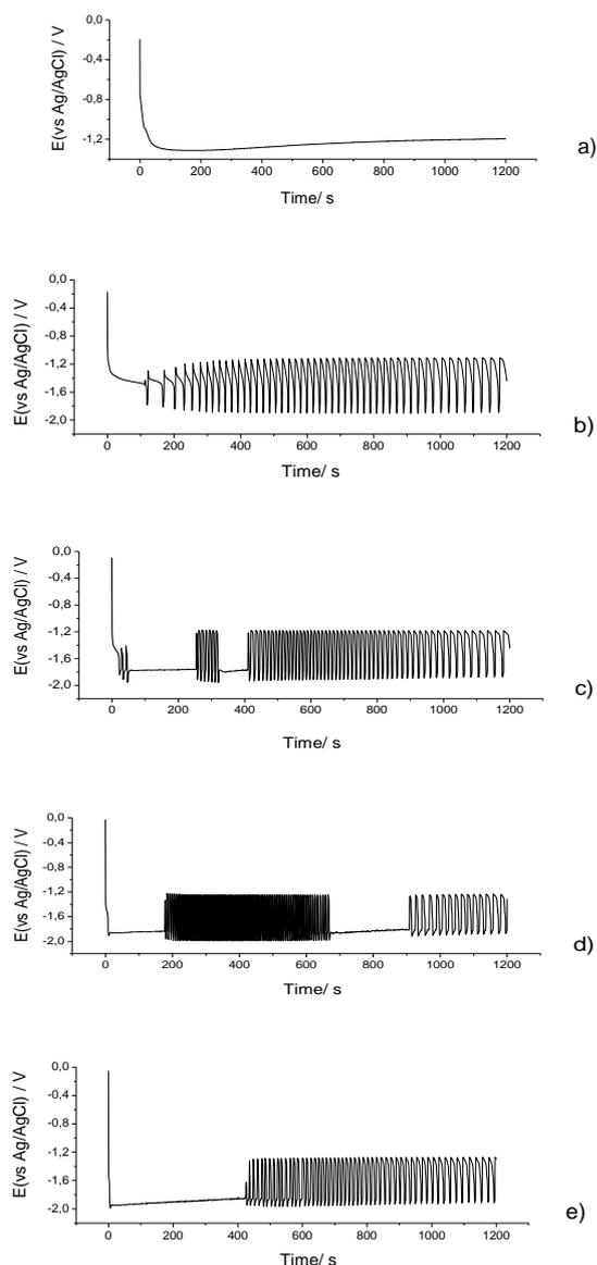
**Fig. 4b.** Chronopotentiometric curves obtained at different current densities at pH=5.  $C_{Sn} = 10 \text{ g dm}^{-3}$ ;  $C_{Co} = 0 \text{ g dm}^{-3}$ . (a)  $0.2 \text{ A dm}^{-2}$ , (b)  $0.4 \text{ A dm}^{-2}$ , (c)  $0.6 \text{ A dm}^{-2}$ , (d)  $1.0 \text{ A dm}^{-2}$ , (e)  $1.4 \text{ A dm}^{-2}$
