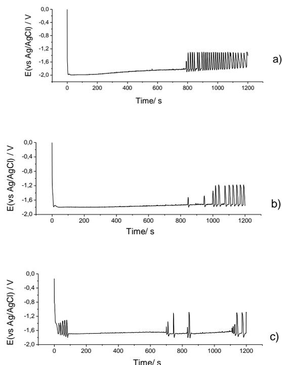
**Fig. 4a.** Chronopotentiometric curves obtained at different current densities at  $\text{pH}=5$ .  $C_{Sn} = 5 \text{ g dm}^{-3}$ ;  $C_{Co} = 0 \text{ g dm}^{-3}$ . (a)  $0.4 \text{ A dm}^{-2}$  (b)  $0.6 \text{ A dm}^{-2}$  (c)  $0.8 \text{ A dm}^{-2}$
