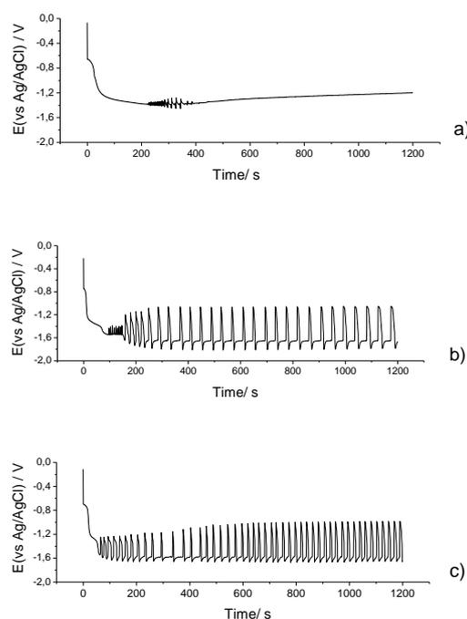
**Fig. 5a.** Chronopotentiometric curves obtained at current densities of  $0.2 \text{ A dm}^{-2}$  at pH=5.  $C_{Sn} = 5 \text{ g dm}^{-3}$ ;  $C_{Co} = 0 \text{ g dm}^{-3}$ . (a)  $\text{C}_{\text{C}_6\text{H}_{11}\text{O}_7\text{Na}} = 50 \text{ g dm}^{-3}$ , (b)  $\text{C}_{\text{C}_6\text{H}_{11}\text{O}_7\text{Na}} = 100 \text{ g dm}^{-3}$ , (c)  $\text{C}_{\text{C}_6\text{H}_{11}\text{O}_7\text{Na}} = 150 \text{ g dm}^{-3}$
