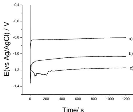
**Fig. 2.** Chronopotentiometric curves obtained at different current densities.  $C_{Co} = 5 \text{ g dm}^{-3}$ ;  $C_{Sn} = 0 \text{ g dm}^{-3}$  (a)  $0.2 \text{ A dm}^{-2}$ , (b)  $0.4 \text{ A dm}^{-2}$ , (c)  $1.4 \text{ A dm}^{-2}$
