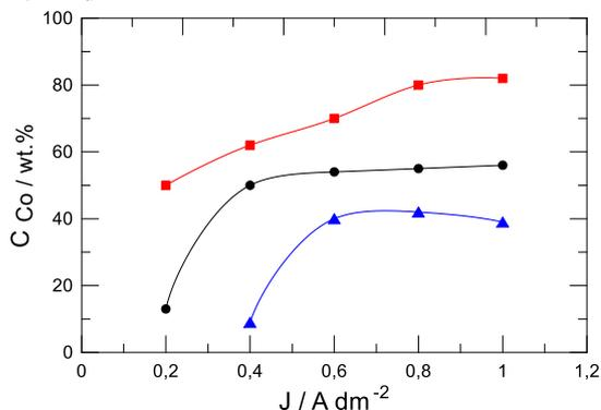
**Fig. 10.** Effect of the current density on the cobalt content in the alloy at different metal concentrations in the electrolyte. ●  $C_{Sn} = 5 \text{ g dm}^{-3}$ ;  $C_{Co} = 5 \text{ g dm}^{-3}$ ; ▲  $C_{Sn} = 10 \text{ g dm}^{-3}$ ;  $C_{Co} = 5 \text{ g dm}^{-3}$ ; ■  $C_{Sn} = 5 \text{ g dm}^{-3}$ ;  $C_{Co} = 10 \text{ g dm}^{-3}$
