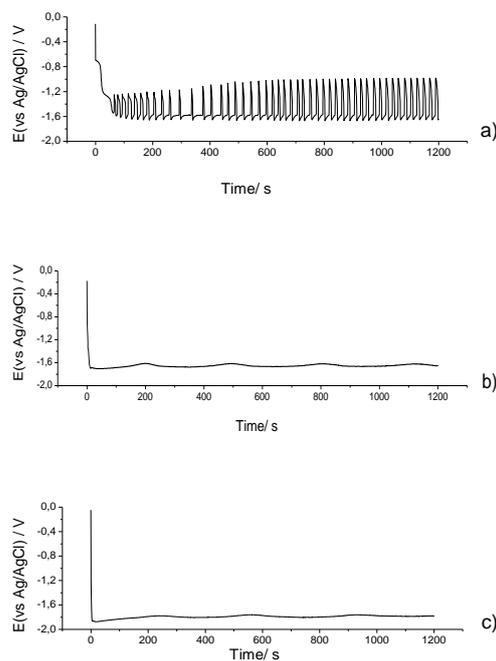
**Fig. 5b.** Chronopotentiometric curves obtained at different current densities at pH=5.  $C_{Sn} = 10 \text{ g dm}^{-3}$ ;  $C_{Co} = 0 \text{ g dm}^{-3}$ ;  $\text{C}_{\text{C}_6\text{H}_{11}\text{O}_7\text{Na}} = 150 \text{ g dm}^{-3}$ . (a)  $0.2 \text{ A dm}^{-2}$ , (b)  $0.4 \text{ A dm}^{-2}$ , (c)  $0.6 \text{ A dm}^{-2}$
