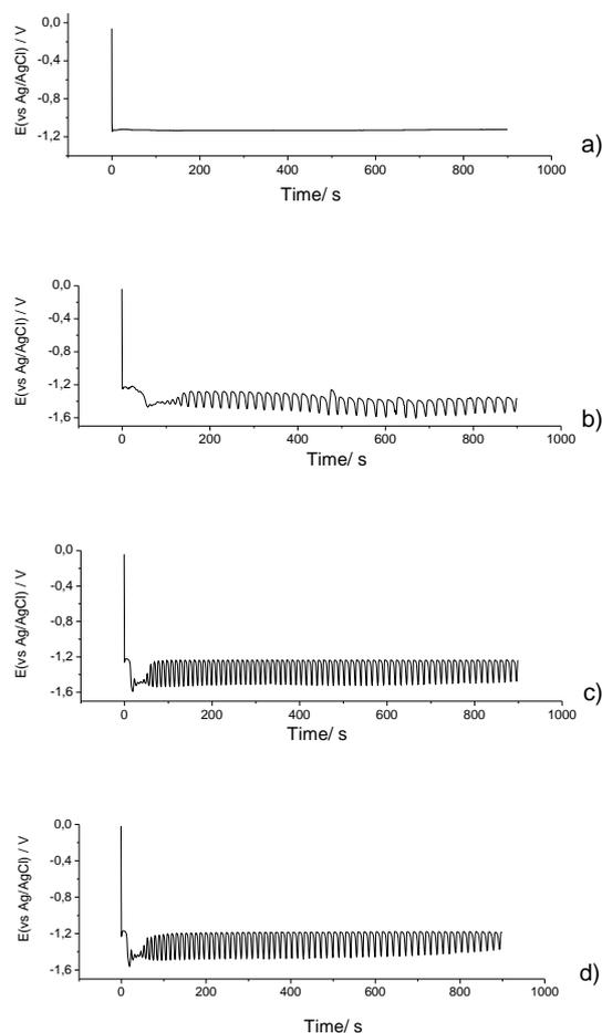
**Fig. 9.** Chronopotentiometric curves obtained at different current densities at pH=5.  $C_{Sn} = 10 \text{ g dm}^{-3}$ ;  $C_{Co} = 5 \text{ g dm}^{-3}$ . (a) 0.6 A dm<sup>-2</sup>, (b) 1.0 A dm<sup>-2</sup>, (c) 1.2 A dm<sup>-2</sup>, (d) 1.4 A dm<sup>-2</sup>
