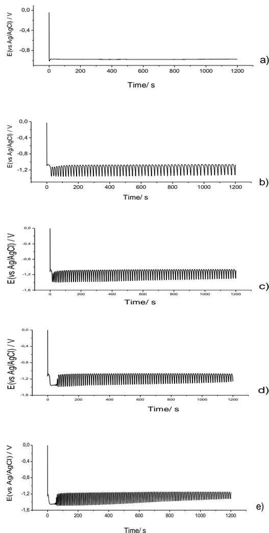
**Fig. 7.** Chronopotentiometric curves obtained at different current densities at  $\text{pH}=5$ .  $C_{Sn} = 5 \text{ g dm}^{-3}$ ;  $C_{Co} = 5 \text{ g dm}^{-3}$ . a)  $0.6 \text{ A dm}^{-2}$ , (b)  $0.8 \text{ A dm}^{-2}$ , (c)  $1.0 \text{ A dm}^{-2}$ , (d)  $1.4 \text{ A dm}^{-2}$ , (e)  $2.0 \text{ A dm}^{-2}$
