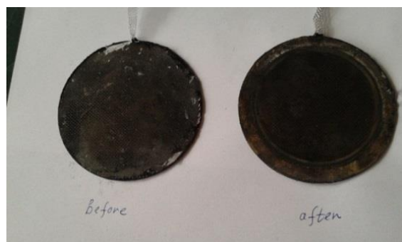
Fig. 10. Gas diffusion electrode before and after 120 C/D cycles.
