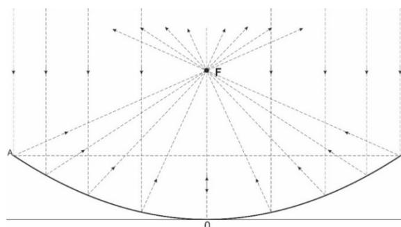
Fig. 2. Principle of action of the solar parabolic cooker (mirror): AB – diameter of the reflector; OF – focal distance.
