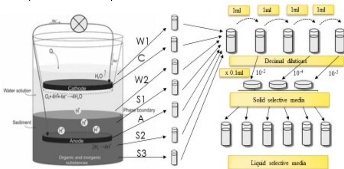
Fig. 1. Scheme of sediment fuel cell and samples' preparation.
