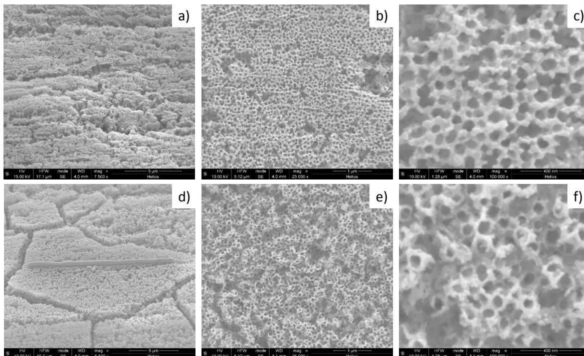
**Fig. 2.** SEM images of the  $\text{FeF}_3$  conversion layers synthesized. The upper row corresponds to the iron substrate, and the lower row to the steel substrate. Magnification increases from left to right. a) 7500x; d) 6500x; b), e) 25000x; c), f) 100000x.
