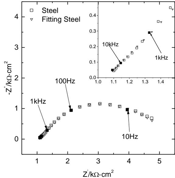
**Fig. 6.** Experimental and fitted impedance data corresponding to the steel sample in Fig. 6. The frequency window was limited to  $f > 1$ Hz. The impedance data were modelled using Eq. 1. The best fitting parameters are collected in Table 3.
