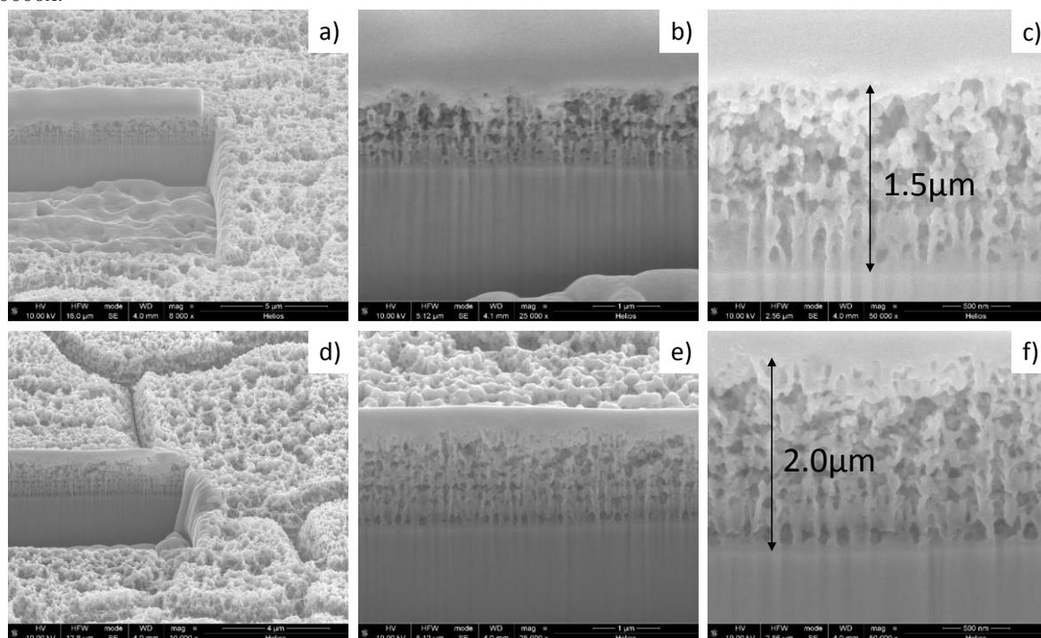
**Fig. 3.** FIB-SEM images of cross sections of the synthesized  $\text{FeF}_3$  coatings. The upper row corresponds to the iron substrate, and the lower row to the steel substrate. (a and d) general view of the section created by  $\text{Ga}^+$  bombardment. (b and e) detail of the layer cross sections with, on top, the Pt layer deposited for conductivity purposes. (c and f) detail of the layer's cross section showing the estimated thickness
