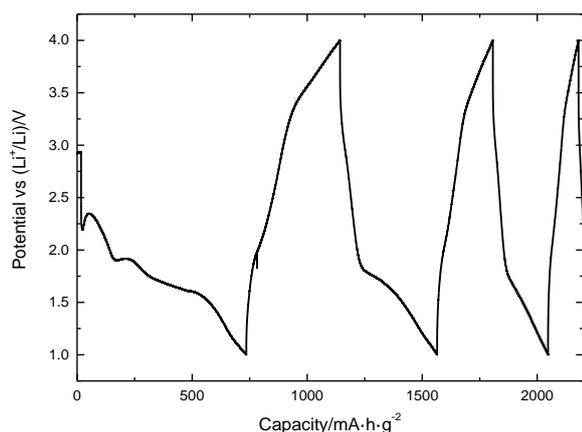
**Fig. 9.** Discharge and charge curves of a  $\text{FeF}_3$  conversion layer grown on mild steel substrate. The electrolyte was 1 M LiBOB salt + 2% FEC in 1:1 EC:DMC. The charge density was calculated assuming cylindrical geometry for the pores (see text).
