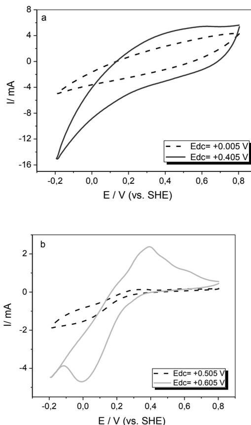
**Fig. 2.** CV of yeast suspension cultivated at applied potentials: a) +0.005 V (dashed line) and +0.405 V (solid line) potentials; b) +0.505 V (dashed line) and +0.605 V (solid line) vs. SHE. Scan rate 10 mV/s.
