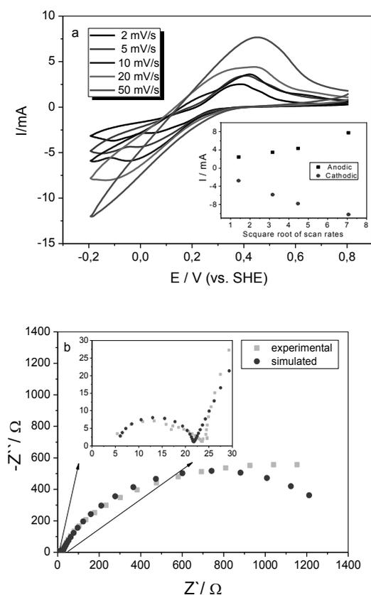
**Fig. 3.** Electrochemical analyses of yeast suspension after chronoamperometric experiments at +0.605 V (vs. SHE): a) CV with different scan rates. Inset: Dependence of anodic and cathodic peak currents on the
