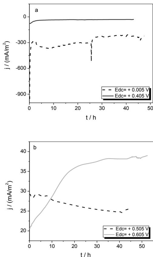
**Fig. 1.** Current densities over time with anodes set at: a) +0.005 V (dashed line) and +0.405 V (solid line) potentials; b) +0.505 V (dashed line) and +0.605 V (solid line) vs. SHE.
