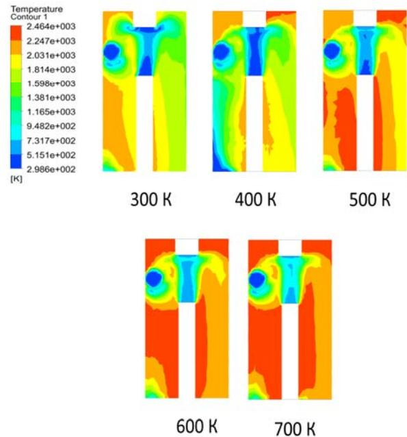
Fig.7. Dependence of temperature on the initial air temperature
