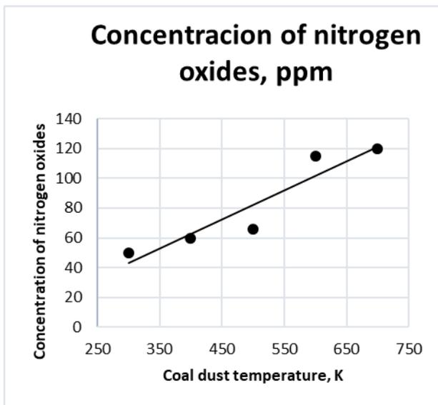
Fig.6. Dependence of concentrations of nitrogen oxides on the temperature of coal dust
