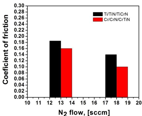
Fig.10. Coefficient of friction in dependence of the N<sub>2</sub> flow
