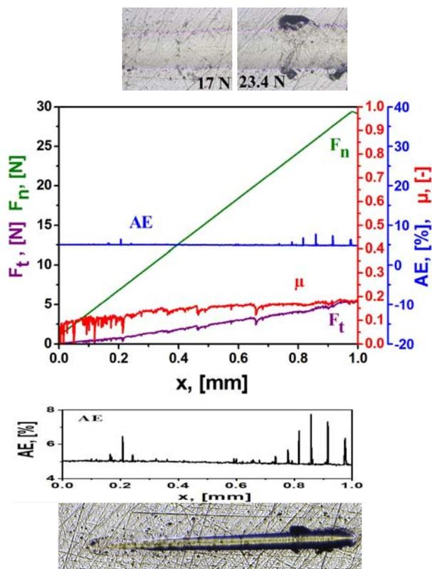
**Fig.6.** Scratch test results for the Ti/TiN/TiCrN coating at 13 sccm nitrogen flow:  $F_n$  - load force;  $F_t$  - friction force;  $\mu$  - coefficient of friction; AE - acoustic emission; and a photo of the scratch test track
