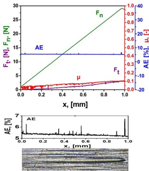
Fig.9. Scratch test results for the Cr/CrN/CrTiN coating at 18 sccm nitrogen flow:  $F_n$  - load force,  $F_t$  - friction force,  $\mu$  - coefficient of friction, AE- acoustic emission; and a photo of the scratch test track
