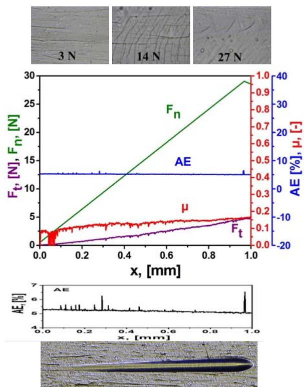
Fig.8. Scratch test results for the Cr/CrN/CrTiN coating at 13 sccm nitrogen flow:  $F_n$  - load force,  $F_t$  - friction force,  $\mu$  - coefficient of friction, AE- acoustic emission; and a photo of the scratch test track
