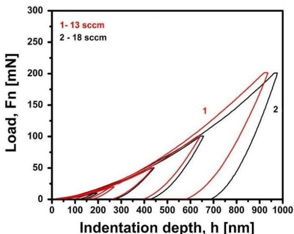
Fig.2. Load-displacement curves for Ti/TiN/TiCrN coating: 1) 13 sccm N<sub>2</sub> flow; 2) 18 sccm N<sub>2</sub> flow
