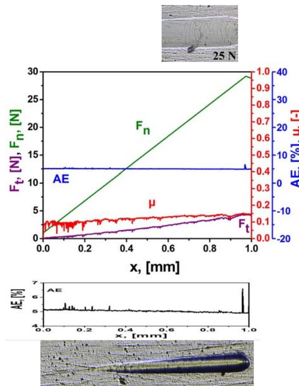
**Fig.7.** Scratch test results for the Ti/TiN/TiCrN coating at 18 sccm nitrogen flow:  $F_n$  - load force,  $F_t$  - friction force,  $\mu$  - coefficient of friction, AE- acoustic emission; and a photo of the scratch test track
