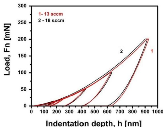
Fig.4. Load-displacement curves for Cr/CrN/CrTiN coating: 1) 13 sccm N<sub>2</sub> flow; 2) 18 sccm N<sub>2</sub> flow
