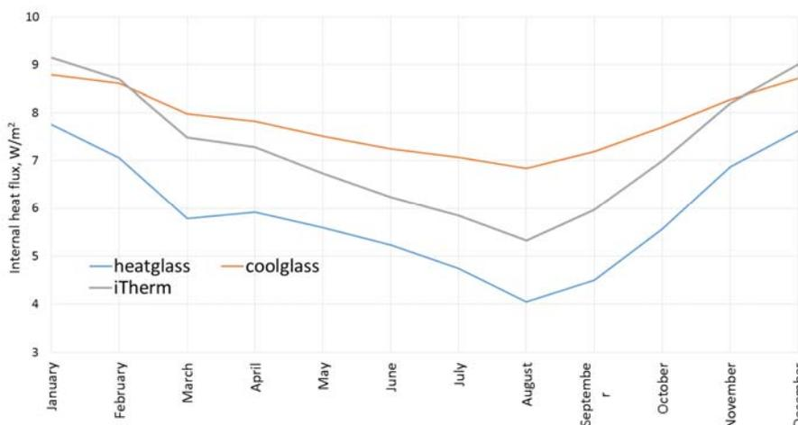
Fig.7. Internal heat flux parameter for the whole year of 2017 year in Sofia.
