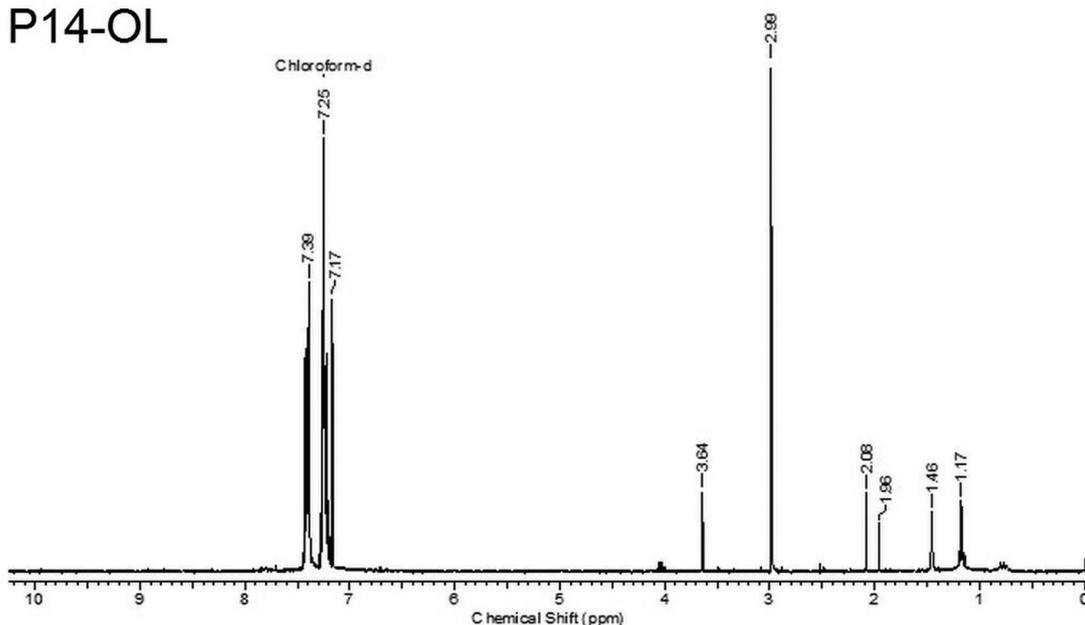
Fig. 4.  $^1\text{H-NMR}$  spectra of polyphenylacetylenes with an olefin end group.
