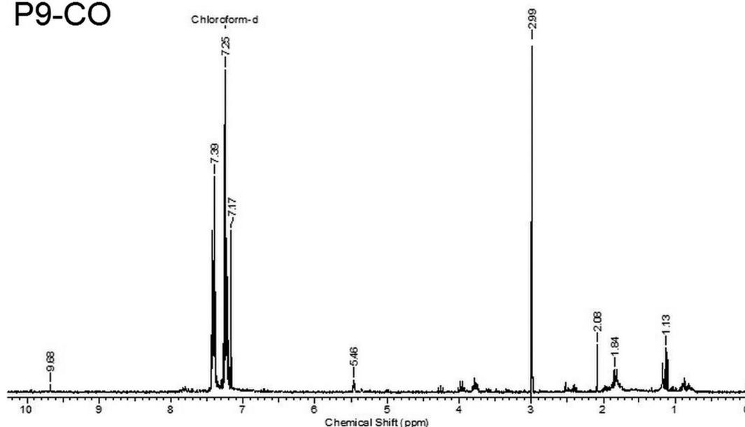
Fig. 3b. <sup>1</sup>H-NMR spectra of polyphenylacetylenes with a carbonyl end group (P7-CO, P9-CO).
