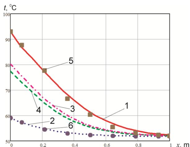
**Fig. 6.** Change of temperatures in a sample of PHE channel at air mass fraction of 55%. Calculated results are presented by solid curves, experimental data by dots. Calculated: 1 – gaseous stream; 2 - cooling water; 3 – liquid film; 4 - wall. Experimental: 5 – gaseous stream; 6 - cooling water.
