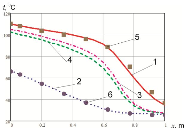
**Fig. 5.** Change of temperatures in a sample of PHE channel at air mass fraction of 3%. Calculated results are presented by solid curves, experimental data by dots. Calculated: 1 – gaseous stream; 2 - cooling water; 3 – liquid film; 4 - wall. Experimental: 5 – gaseous stream; 6 - cooling water.
