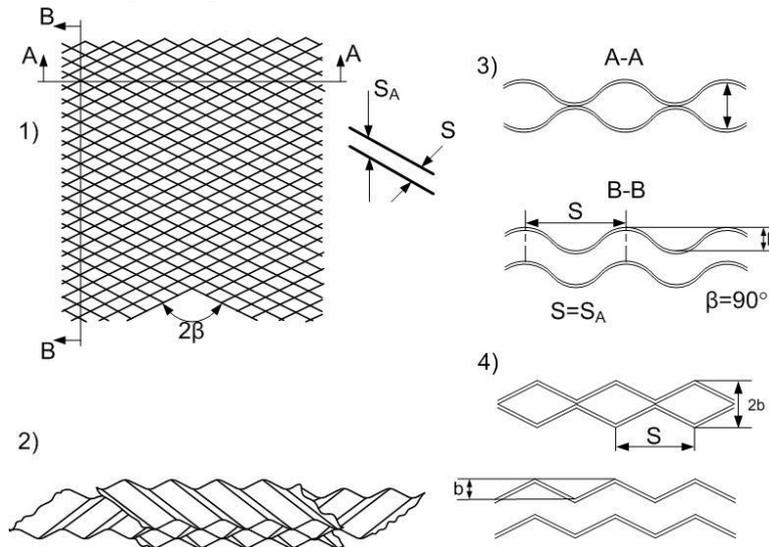
**Fig. 3.** Different corrugation forms: 1, 2 –intersection of the adjacent plates; 3 – channel cross-sections for the sinusoidal form of corrugations; 4 – channel cross-sections for the triangular form of corrugations.
