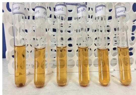
**Fig. 5.** Effect of nickel nitrate solution concentration on nickel nanoparticles synthesis by *T.brevifolia* extract (pH of the solution was 8, 2 ml of the *T.brevifolia* extract, time: 30 min, stirring rate 150 rpm)
