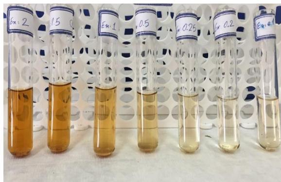
**Fig. 4.** Effect of *T.brevifolia* extract solution on nickel nanoparticles synthesis (pH of the solution was 8, 5 ml of 0.001 M nickel nitrate, time: 30 min, stirring rate 150 rpm)
