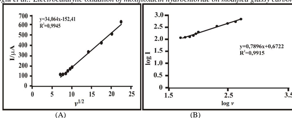
**Fig. 6.** (A) The peak current values plotted against  $\nu^{1/2}$  and (B) the logarithm of peak current ( $\log I$ ) against the logarithm of scan rate ( $\log \nu$ ) of the oxidation peak obtained from the CV voltammograms recorded at the poly(4-ABSA/GC) electrode of  $1 \times 10^{-4}$  M MOX in 0.2 M acetate buffer (pH 5.0) (scan rates: a) 50, b) 60, c) 70, d) 80, e) 90, f) 100, g) 200, h) 300, i) 400, j) 500  $\text{mV s}^{-1}$ ).
