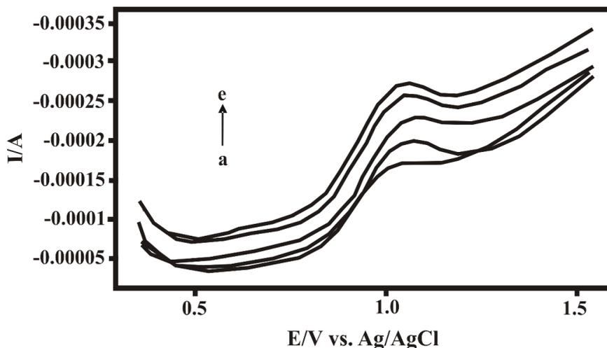
**Fig. 8.** DPV voltammograms for increasing concentrations of MOX: a)  $1 \times 10^{-6}$ , b)  $3 \times 10^{-6}$ , c)  $5 \times 10^{-6}$ , d)  $7 \times 10^{-6}$  and e)  $9 \times 10^{-6}$  M in the potential range from 0.2 V to 1.4 V in 0.2 M acetate buffer (pH 5.0) on the poly(4-ABSA/GC) electrode surface.
