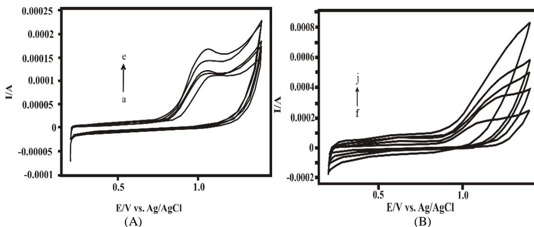
**Fig. 5.** Cyclic voltammograms recorded at the poly(4-ABSA/GC) electrode in 0.2 M acetate buffer (pH 5.0) containing  $1 \times 10^{-4}$  M MOX (scan rates: (A) a) 50, b) 60, c) 70, d) 80, e) 90 and (B) f) 100, g) 200, h) 300, i) 400, j) 500 mV s<sup>-1</sup>).
