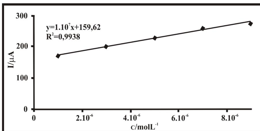
**Fig. 9.** Calibration plot for increasing concentrations of MOX obtained from DPV voltammograms.
