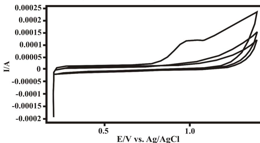
**Fig. 7.** The cyclic voltammogram of three cycles recorded in the potential range from 0.2 to 1.4 V of  $1 \times 10^{-4}$  M MOX in 0.2 M acetate buffer (pH 5.0) at the poly (4-ABSA/GC) electrode (scan rate:  $50 \text{ mV s}^{-1}$ ).
