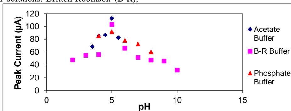
Fig. 4. The oxidation peak current values of 1×10<sup>-4</sup> M MOX recorded in the range from pH 2.0 to 10.0 in 0.1 M phosphate, 0.04 M B-R and 0.2 M acetate buffers (scan rate: 50 mV s<sup>-1</sup>).
