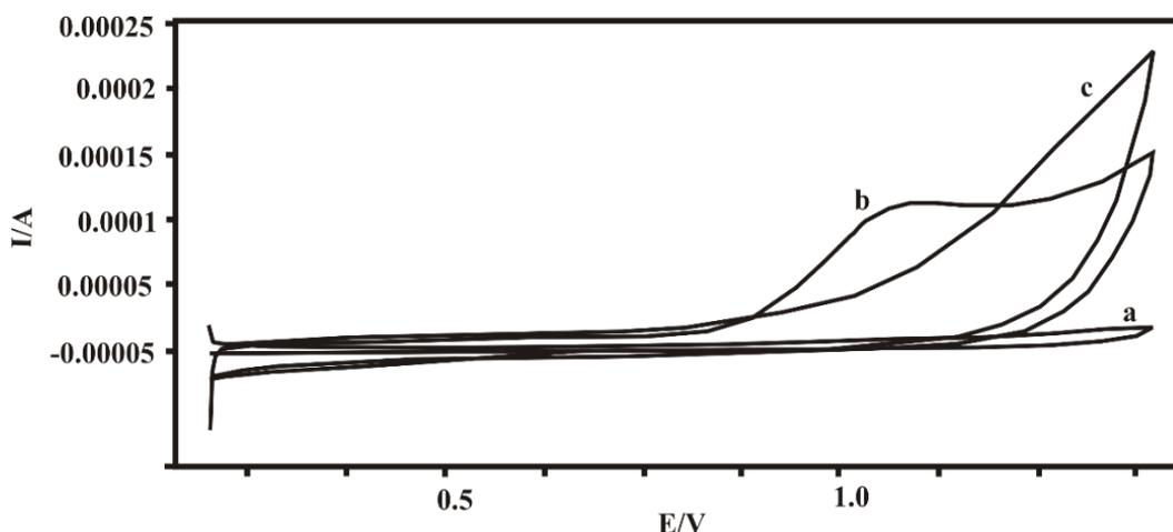
Fig. 3. Cyclic voltammograms of  $1 \times 10^{-4}$  M MOX recorded at the bare GC (a) and poly(4-ABSA/GC) (b) electrodes in 0.2 M acetate buffer (pH 5.0). The voltammogram of 0.2 M acetate buffer (pH 5.0) (c) is the background obtained by using the modified glassy carbon (scan rate:  $50 \text{ mV s}^{-1}$ ).
