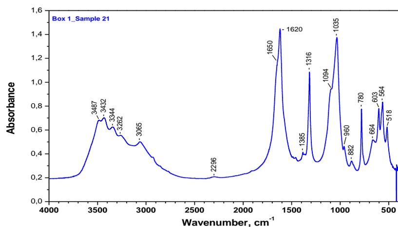
Figure 4. FTIR spectra of calcium oxalate monohydrate and  $\text{Ca}_5(\text{PO}_4)_3 \text{OH}$
