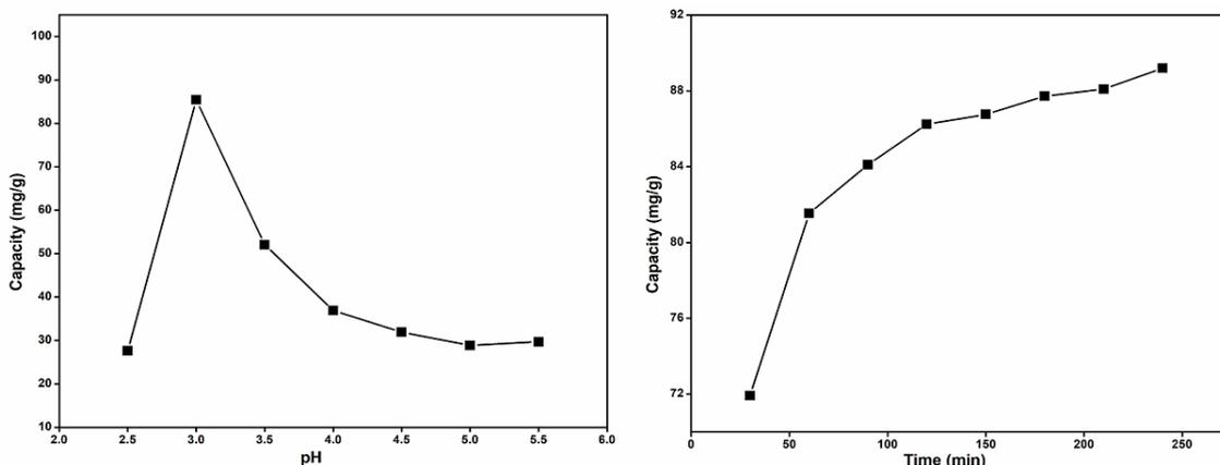
**Figure 5.** Effect of pH and time on chromium adsorption.
