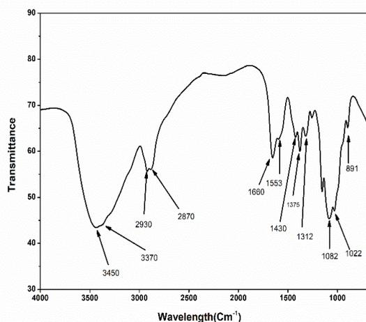
Figure 1. FTIR spectrum of the chitosan film
