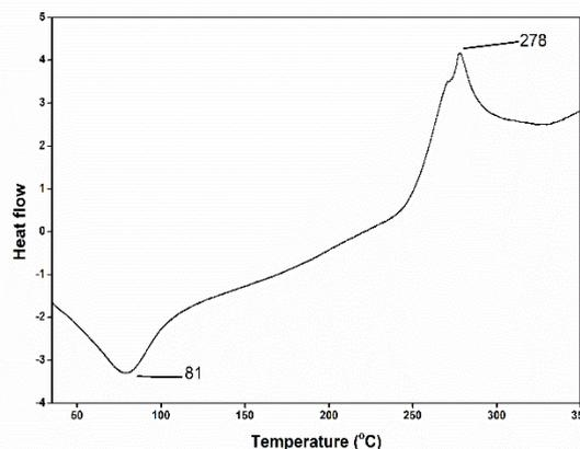
Figure 3. DSC curve of chitosan.
