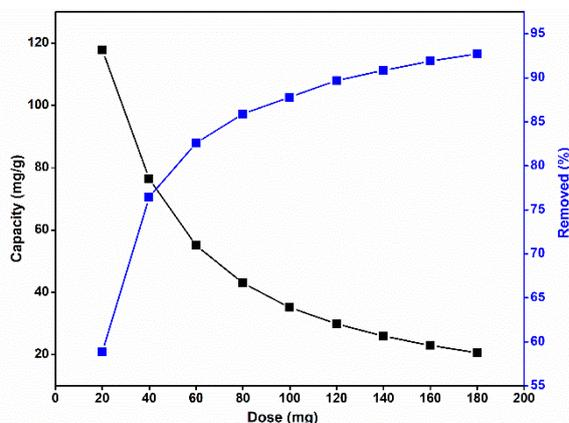
**Figure 4.** Effect of sorbent dose on chromium adsorption.
