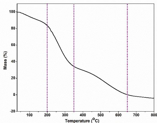
Figure 2. TGA curve of chitosan.
