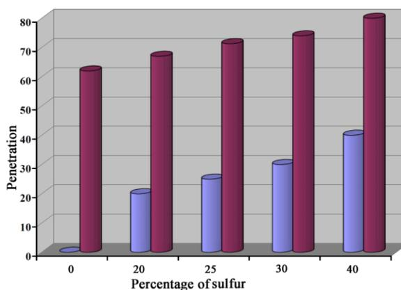
**Figure 6.** Penetration diagram of bitumen after addition of sulfur.
