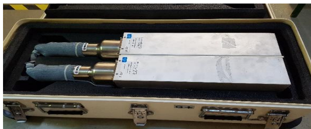
Fig. 1. Opened detector protection box, keeping a pair of NaI(Tl) detectors used in the survey.
